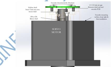
After coupling the encoder hollow shaft with the rigid motor shaft, always fasten attached screws securely. Be sure to firmly tighten two hex-screws that located at encoder' s hollow shaft, apply threads-lock glue and tightly screwed in for long-term use. Also follow above procedures for the encoder M3 screws when mounting the encoder onto servo motor.
